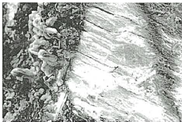
Figure 10-2. Wood damaged by white rot is fibrous, spongy and bleached.
