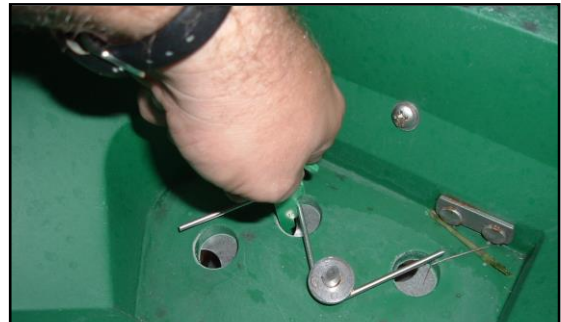
Figure 2. Place calibration step key placed in the center hole to calibrate spreader
